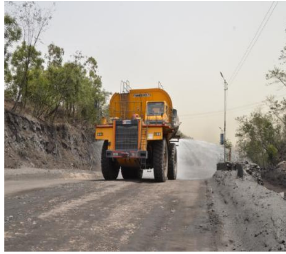
70 kl water sprinkler for mine haul road
