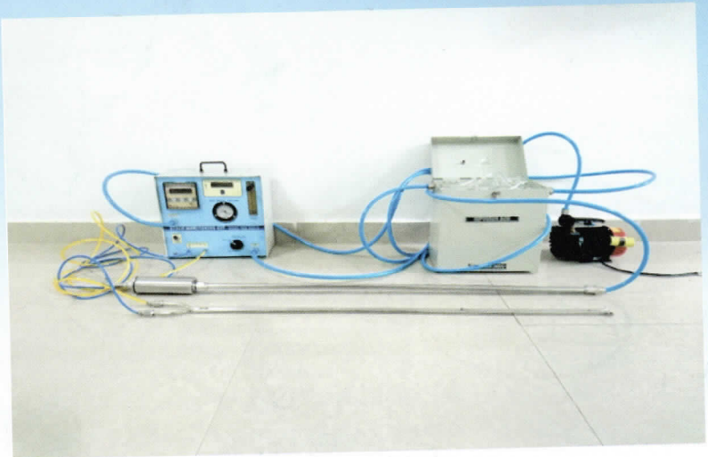
Emission Monitoring Equipment
